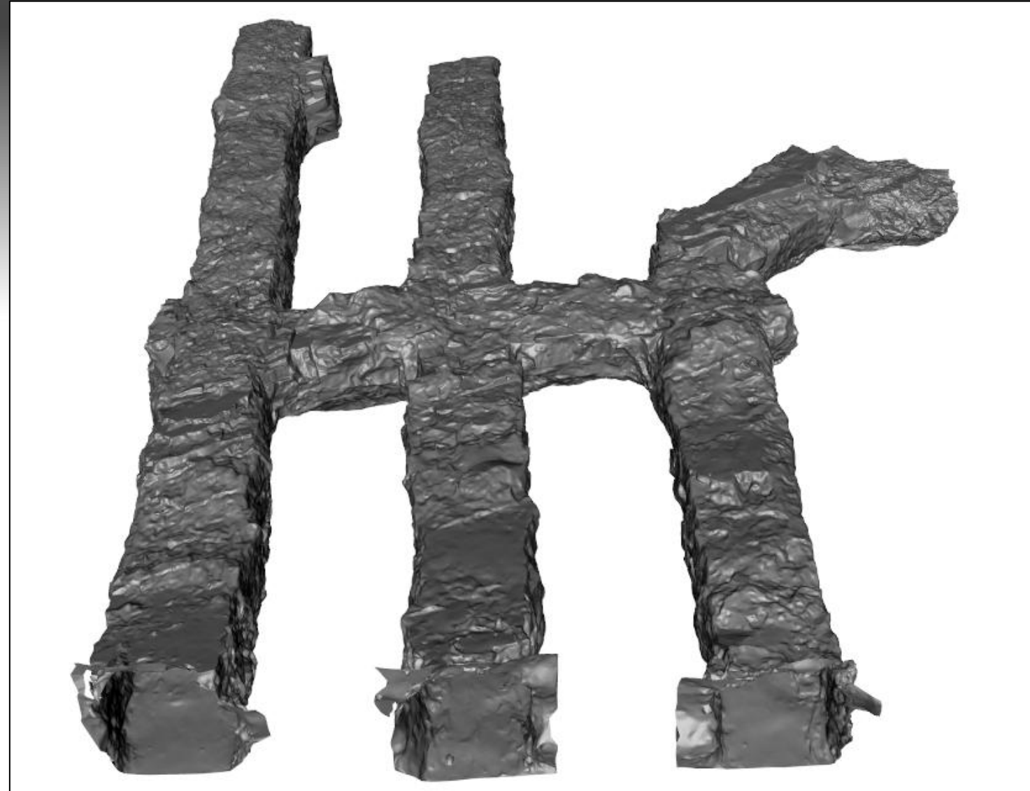
3D MODEL CONSTRUCTED FROM LIDAR POINT CLOUDS
